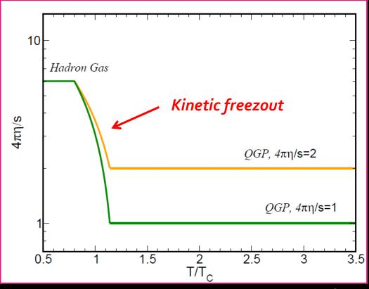
A **smooth kinetic freezout** is implemented in order to gradually reduce the strength of the interactions as the temperature decreases below the critical temperature.
