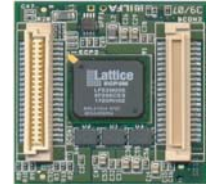
Optical End Point: back view Board: (4.0 cm x 4.5 cm)
