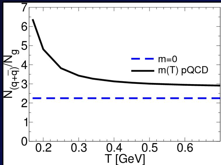
$$\frac{N_{q+\bar{q}}}{N_g} = \frac{d_{q+\bar{q}}}{d_g} \frac{m_q^2(T) K_2(m_q/T)}{m_g^2(T) K_2(m_g/T)}$$
